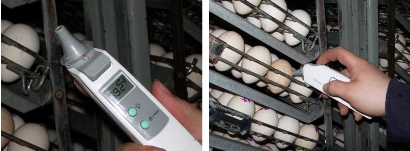
Figure 1: IR ear thermometer for egg surface temperature measurement
